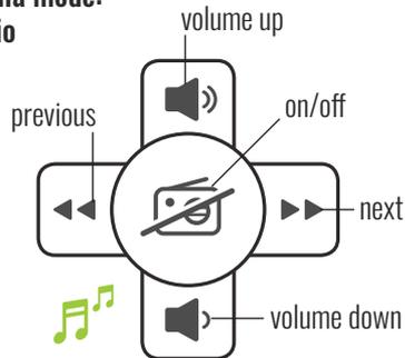
Media mode is available when the boat has a media package installed. Media mode allows you to control the music playing through the radio.
