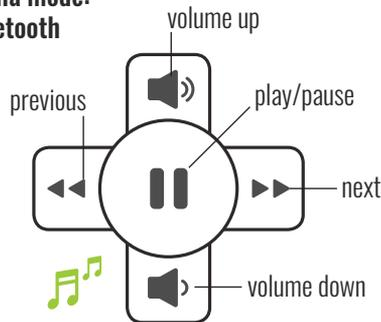
When you stream music from a Bluetooth paired smartphone, media mode controls switch through audio tracks instead of radio channels.
