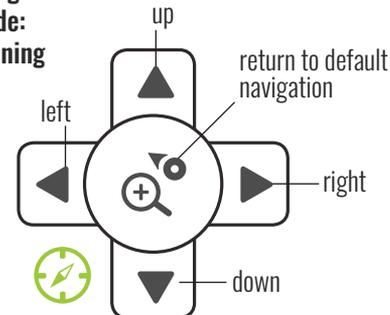
You can switch between default and panning navigation mode by pressing the center key.
